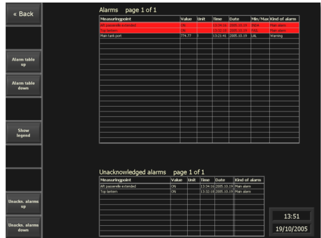
A list of all alarm messages including when the alarm was triggered, the corresponding measured value and the type of alarm (warning or main alarm).
